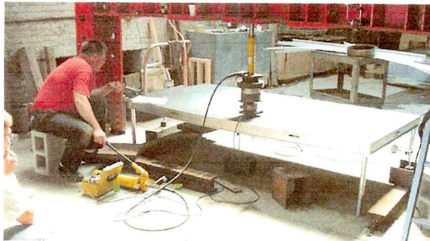
Concentrated load test
