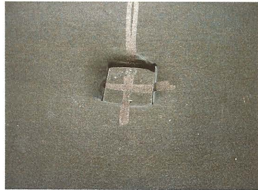
Imprint on test surface caused by load plate
