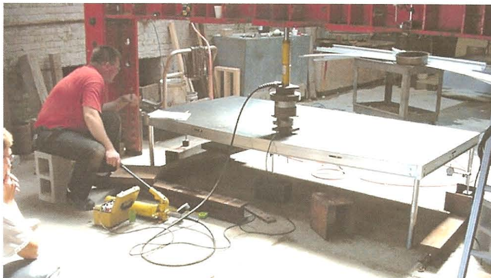
Concentrated load test
