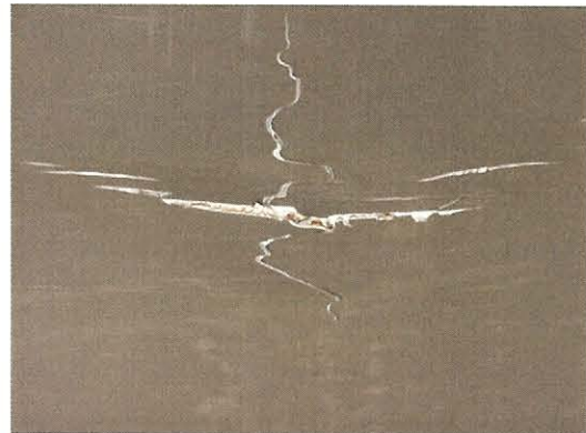
Deformation of lower surface after concentrated loading
