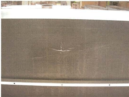
Deformation of lower surface after concentrated loading
